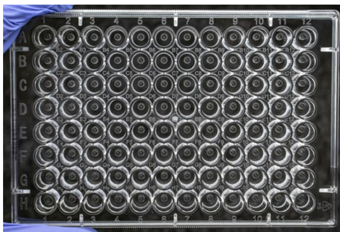
Figure 1. Droplets of Corning Pluronic sacrificial ink without cells dispensed in a 96-well microplate, using the parameters in Table 1.
