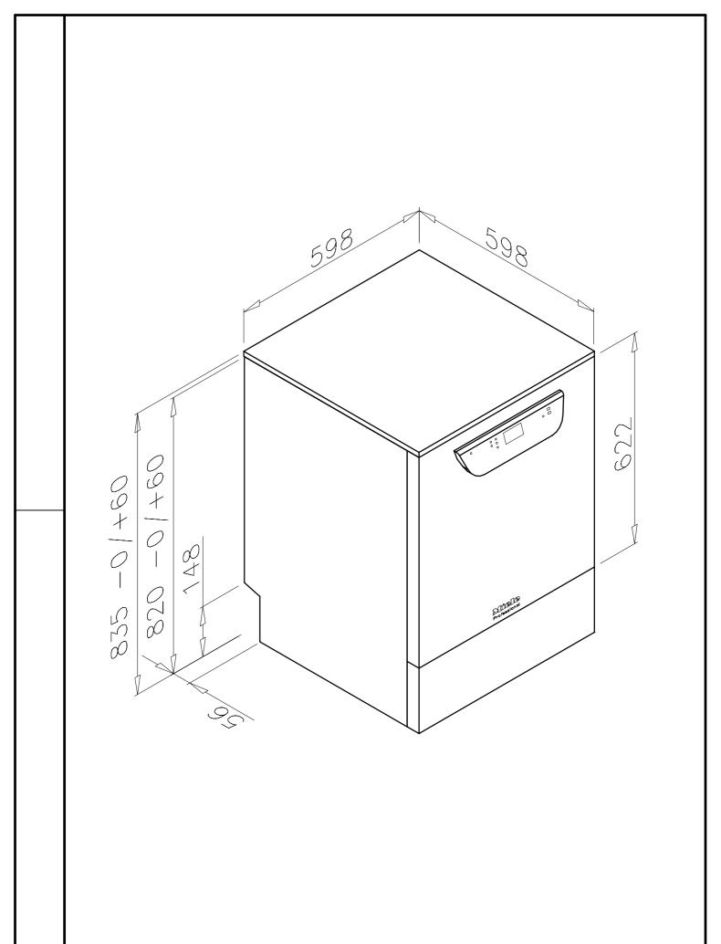
Míele PROFESSIONAL Installationsplan/Installation plan Thermo—Desinfektor PG 8591 — PG 8593
